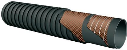
**APPLICATION** For suction and delivery of oils, diesel fuel, petrols and petroleum products. Recommended in applications where reduced bending radius is required. Extensive application in the automotive and industrial vehicles sector as multipurpose flexible hose.
