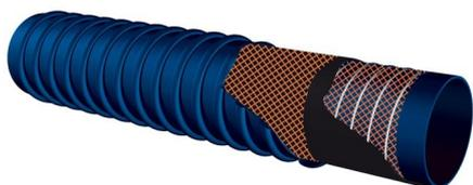
**APPLICATION** Flexible hose for the passage of cooling water and exhaust gas of combustion engines of water-crafts and ships. In compliance with SAE J2006 R2 MARINE EXHAUST HOSE Standard.
