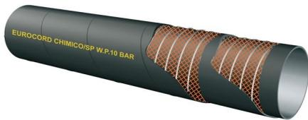
**APPLICATION** Suction and delivery of solvents organic and inorganic acids, salts, basis, ketones at high concentration. Double spiral guarantees particular flexibility thus making this hose very easy to handle and allowing exceptionally narrow bending radius.
