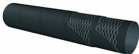
**APPLICATION** Conveyance of diesel fuels and unleaded petrol in watercrafts and ships. Extremely lightweight and flexible pipe with very good bending radius. In compliance with EN ISO 7840-A1 - 1994. R.I.NA and LLOYD'S Standard.
