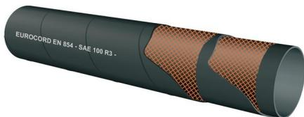
**APPLICATION** Delivery of hydraulic fluids, mineral oils, lubricants, diesel fuel. In compliance with SAE J 517 100R6/EN 854 type R3 Standard.
