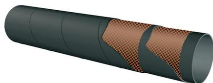
**APPLICATION** Conveyance of diesel fuels and unleaded petrol in watercrafts and ships. Particularly used for heavy-duty applications. Its main features are light-weight and flexibility. In compliance with EN ISO 7840-A1 - 1994. CE 0474 R.I.NA and LLOYD'S Standard.
