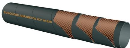
**APPLICATION** For low pressure transport of abrasive products and fluids in general, especially liquid cement, plaster, grout, gypsum, sand. It is supplied together with high pressure pumps or peristaltic pumps.
