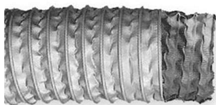
**APPLICATION** Extremely flexible and lightweight hose produced with polyamide fabric PVC coated on both sides and built-in harmonic steel PVC coated spiral. Suitable for air, fumes and dust passage. Particularly recommended for the civil and ship air-conditioning sector.
