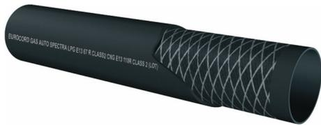
**APPLICATION** Suitable for low pressure delivery of liquefied gas in gaseous state in car kit. Its lightweight and flexibility features make assembly in narrow spaces easier. Specifications are in compliance with ECE Reg. 110.00 class 2 and ECE R67.01 class 2 Standard.
