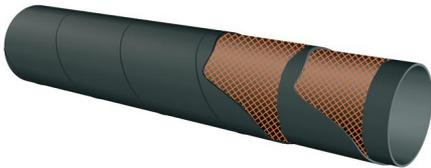
**APPLICATION** For pneumatic or electric vibrators, for leveling concrete shuttering. The rubber adopted gives this hose exceptional tensile elongation characteristics. Its particularly thickened structure allows to avoid creation of cusps also in cases of very narrow bending radius.
