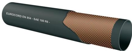
**APPLICATION** Delivery of hydraulic fluids, mineral oils, lubricants, diesel fuel. In compliance with SAE J 517 100R6/EN 854 type R6 Standard.
